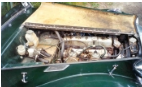
Triumph six is shoehorned along with a couple of carburetors into the narrow Almac engine bay.
