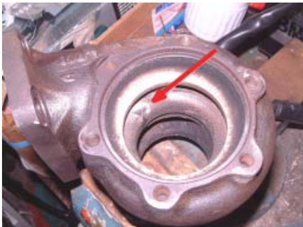
Cracked exhaust housing - (crack indicated)
