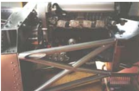
Construction method note the use of angle extrusion between sheet face
