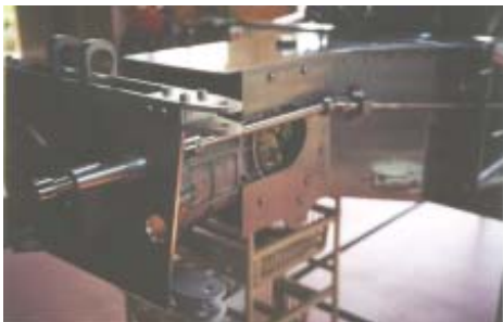
Fabricated bellhousing and rear bulkhead
