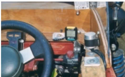
Close up of hi-tech bicycle speedo. The lever beside the speedo says hood and opens just that.
